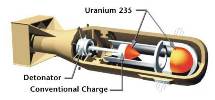
One piece of <sup>235</sup>U was fired into a second piece of <sup>235</sup>U, with the two combined pieces exceeding the *critical mass* required for *sustained nuclear fission* to take place.
