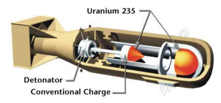
"Little Boy" contained approximately 50 kg of enriched <sup>235</sup>U, which was detonated by a gun-type mechanism.
