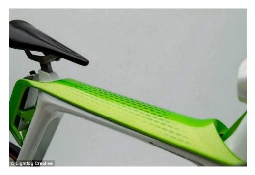
• The unusual-looking green frame is designed to convert sunlight into energy that would power the bike's battery and consequently the filter system.
