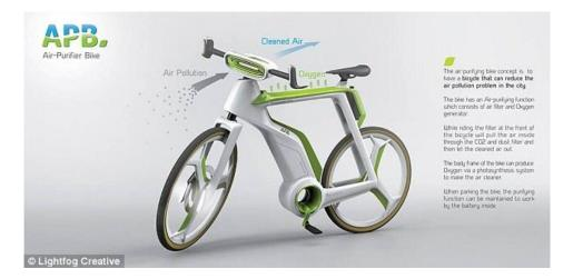
• It concept design comprises an air filter that screens dust and pollutants from the air, a photosynthesis system (including a water tank) that produces oxygen, an electric motor and a battery, the company said.
