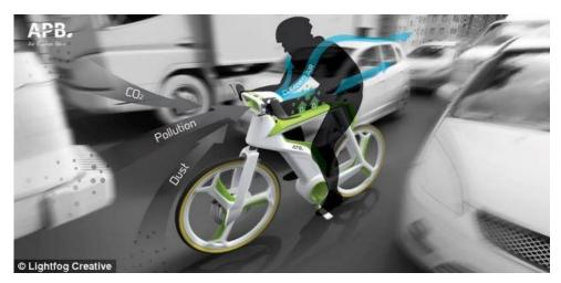
• The bike is designed so that when it is being ridden, air passes through the filter fixed between the handlebars, where it is cleaned before being released toward cyclist.
