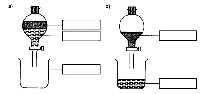
c) Oil and water are two immiscible liquids, *i.e.* they do not mix with each other. The less dense oil floats on the surface of the more dense water. The stopper is removed from the separating funnel, and then the tap is opened. Water (the bottom layer) will flow into the beaker. Just as the layer of oil reaches the tap, the tap is closed, leaving the water in the beaker and the oil in the separating funnel.
