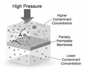
• Diagram showing the process of reverse osmosis. A high pressure is applied to water that is contaminated with impurities. Only water molecules are small enough to be forced through the partially permeable membrane, creating water that is low in contamination and suitable for drinking.
