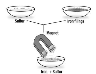
b) In the example given above, iron is a magnetic material and is attracted towards the magnet, while sulfur is not a magnetic material and is not attracted towards the magnet. Iron filings are attracted towards the magnet and separated from the sulfur which remains behind in the dish.
