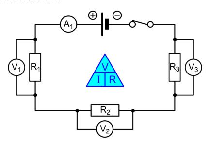
• Battery = 12 V •  $R_1 = 20 \Omega$  •  $R_2 = 50 \Omega$  •  $R_3 = 80 \Omega$
